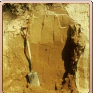
Soil properties used to assess soil suitability for onsite wastewater treatment include the presence or absence of redoximorphic features (color patterns in soil formed by repeated oxidation and reduction of iron and manganese) that indicate wetness in soils. These pictures show (top) well-drained sandy soil with no limiting factors, (middle) red splotches near the shovel blade indicating moderate seasonal wetness, and (bottom) redoximorphic color patterns indicating a very wet soil.
