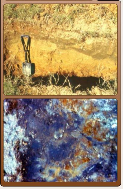
As effluent from a drainfield passes through a silty soil, particulates are filtered out in a relatively short distance. Most bacteria, viruses, or other potential disease-causing organisms cannot pass through long distances of dry soil; they remain within the first few feet. In saturated soils, organisms may travel greater distances. Water moves very slowly through soils with high clay content, and consequently, clay soils require a large area in order to treat the effluent.
