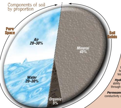
cles, organic particles, water, and air. See the figure below for a simple pie chart representing these proportions. Note that only about half of the soil volume consists of solid material. The other half consists of pore spaces filled with air or water.
