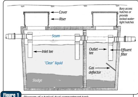
Diagram of a typical dual compartment tank.
