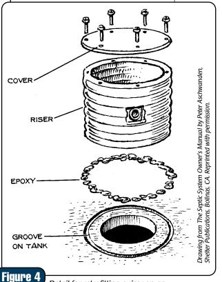
Detail for retrofitting a riser on an existing tank.
